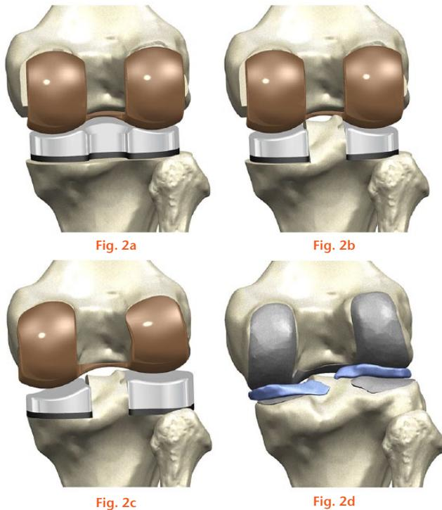
FEM used in analysis: a) standard off-the-shelf cruciate-retaining total knee arthroplasty (TKA); b) standard off-the-shelf bicruciate-retaining TKA; c) patient-specific bicruciate-retaining TKA; d) normal adult knee.
