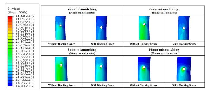
Fig c. Stress distribution on the cortical bone (around distal locking screw hole) of finite element model.
