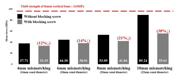
**Fig d.** Mean stress over a region of interest on the cortical bone (around distal locking screw hole) in each finite element model and reduction rate of the mean stress by using a blocking screw in each model. MPa, megapascal.
