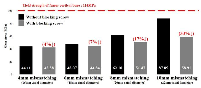
**Fig b.** Mean stress over a region of interest on the cortical bone (around lag screw hole) in each finite element model and reduction rate of the mean stress by using a blocking screw in each model. MPa, megapascal.
