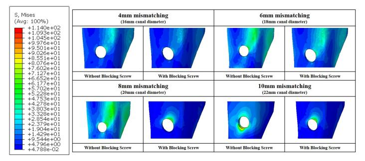
Fig a. Stress distribution on the cortical bone (around lag screw hole) of finite element model.
